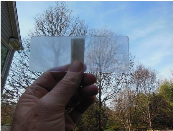
Transmission was increased by 40% over the control after transcrystallinity. Percent Crystallinity significantly increased epitaxial to the plane of crystal growth making the surface properties harder and less prone to surface oxidation or staining.
