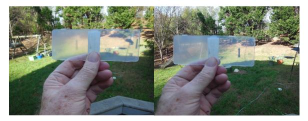
Plaques on left is the Control Pinnacle 5110C3 and Sample on the right the same resin with induced trans-crystallinity under identical molding and cooling conditions.
